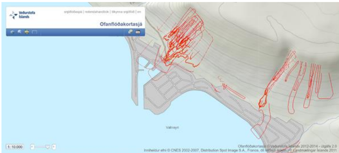
Figure 2.2: Map of avalanche paths in Patreksfjörður. The recorded avalanche paths are marked by the red lines. (Modified from IMO, 2021a)
